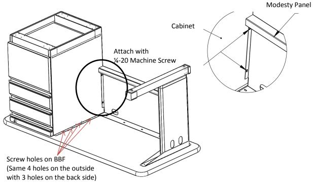
**Step 3B**: (If your Ped contains totes): Remove all totes from the ped. Place your Tote Ped upside down on the top opposite the leg. Align the modesty panel to with the Ped and the Leg. Attach to the Ped and the leg with (4) ¼-20 Screws.
