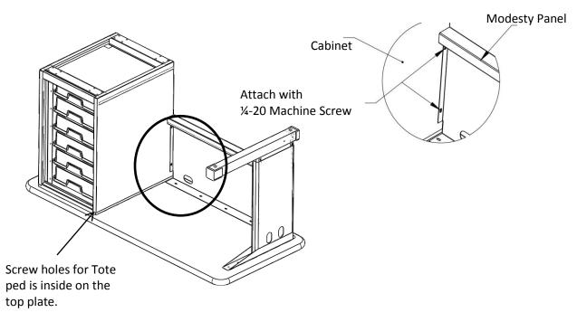
**Step 4**: Attach the Cascade Ped and modesty panel to the table top using the supplied wood screws. Hole placement for the Peds are shown in the previous step.
