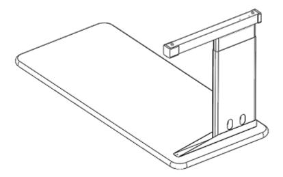
**Step 2**: Adjust the legs to the desired height by taking out the (4) ¼-20X1/2" Machine screws per leg and reinserting them at the desired height.
