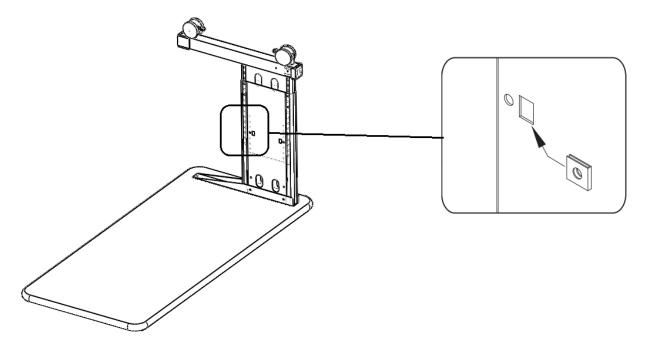
**Step 3A**: (If your Ped is a Box Box File): Place the Box Box File (BBF) upside down on the table top opposite the leg. Align the Modesty Panel with the two holes on the BBF and the leg, attach to the BBF and the leg using (4) ¼-20 Machine Screws. The screw holes on the BBF are along the outside of the top plate (as seen in the picture).
