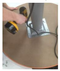
Step 4: If equipped with power, pass power cords through base as shown.
